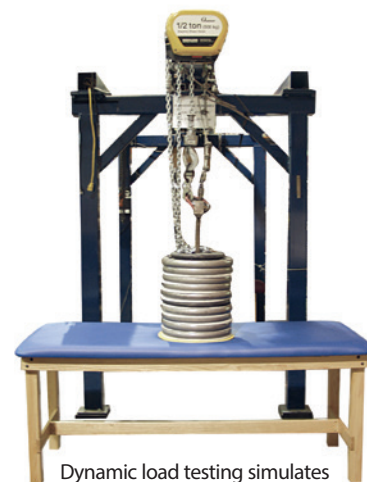
Dynamic load testing simulates real-life hop and drop table use.
